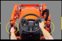
Step 2: Unlatch the loader latch levers to detach the front loader hooks.
