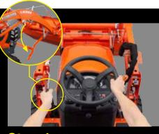
Lift the loader boom and fully dump the bucket. Pull stand release lever to lower the front loader stand.
