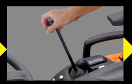
Step 3: Use the loader lever to remove the loader frame from the mast.
