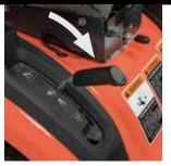
Release the lever to lower the deck
