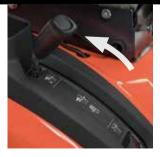
Pull the lever to lift the deck
