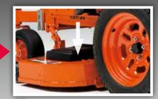
Push and release the pedal again to lower the deck
