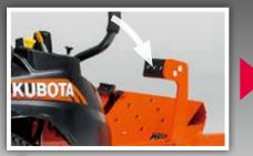
Push and release the pedal to raise the deck
